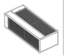
For a further energy-saving, the MEHITS conditioners are equipped with a proportional automatic free-cooling system in order to obtain free cooling when the indoor temperature is higher than outdoor one. Practically, the fresh air is used as coolant, when the outside conditions allow for this, in order to cool the ambient.
