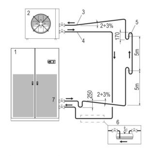
REALIZE THE REFRIGERANT LINE WITH THE INDICATED INCLINATIONS TO EASE THE RETURN TO THE COMPRESSOR OF THE LUBRICANT OIL
