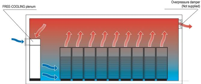
The plenums have same technical characteristics and base dimensions of the machine cabinet. The optional allow to obtain free-cooling by direct ambient air intake into the room.
